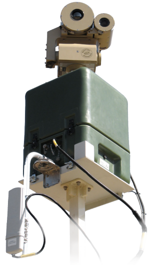
Radar detects, camera assesses
